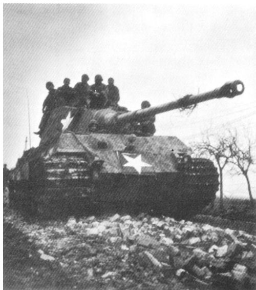
CAPTURED GERMAN TIGER (MARK VI) TANK with temporary U.S. markings. Note 88-mm. gun with flash hider.
