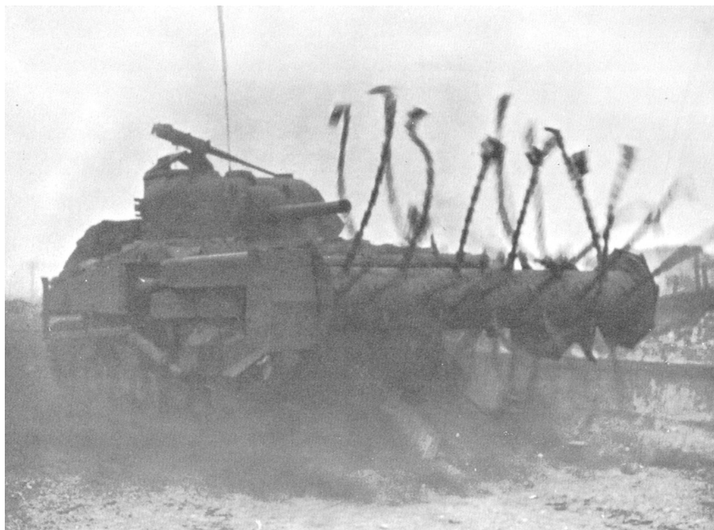
BRITISH FLAIL TANK beating the road to explode mines.
